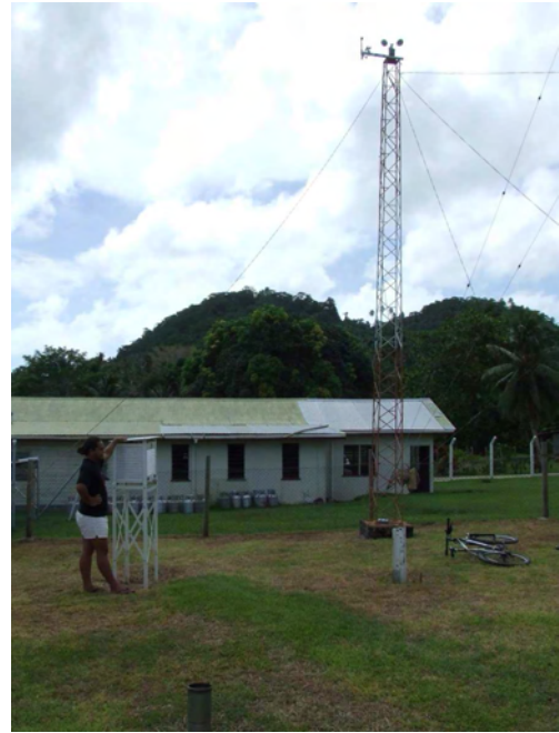
(b) Ten meter mast at the Ahau government station. The equipment was mounted on top of the existing ten meter mast belonging to the weather station.
